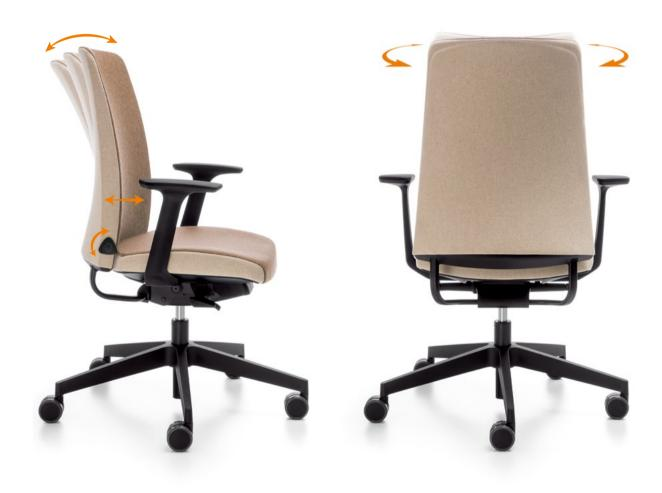
Specially designed frame covered with cold molded foam makes the back support extremely flexible and allows for dynamic adjustment to the user's body. Lumbar support fully integrated into the backrest (schukra) allows a precise adjustment of the chair shape to the user's needs.
