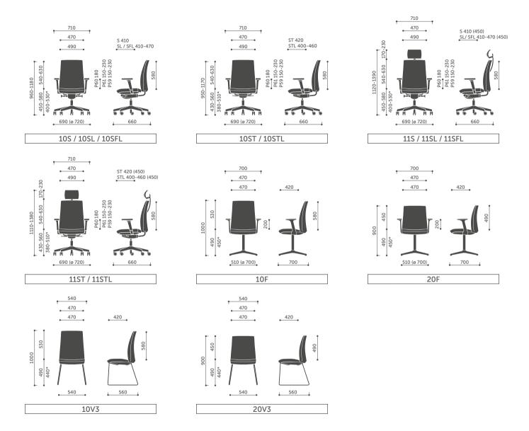
$<sup>^{*}</sup>$ Seat height is measured according to PN EN 1335-1 norm (with seat burden).
